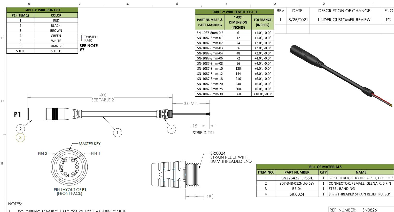
SOLDERING IAW IPC-J-STD-001 CLASS II AS APPLICABLE. CABLE ASSEMBLIES TO BE TESTED 100% FOR CONTINUITY AND SHORTS.
