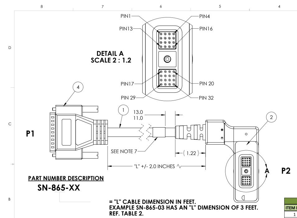
**BILL OF MATERIALS** ITEM NO. PART NUMBER QTY **NAME COMMENTS** 51367  $\mathsf{AR}$ WIRE 32C CABLE INCLUDES HOUSING, FASTENERS, 2 TE-32M-ASSY 2 **CONNECTOR ASSEMBLY** THUMBWHEEL. PROVIDED BY **SUPPLYNET** 3 DB44 MALE **INDUSTRY STANDARD** TBD 1 4 SN0057 1 PCB SUPPLYNET PROVIDED.
